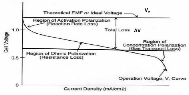
Voltage current density characteristics Polarization curve
