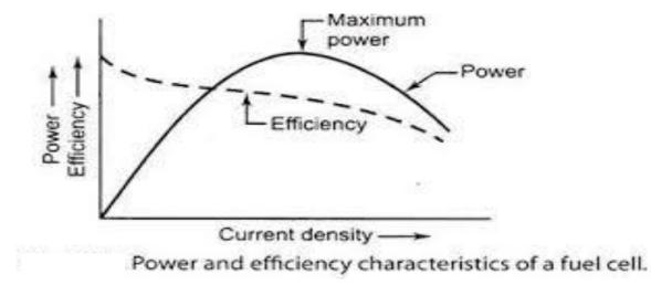
The power loss is converted to west heat and released to atmosphere. After reaching saturation the power per cell starts decreasing. The losses increase and are converted to waste heat.
