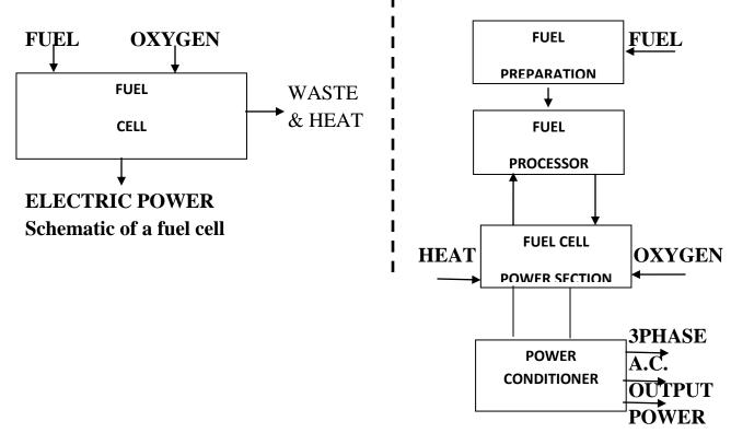
Schematic of a fuel cell power plant
