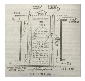
Continuous operation requires the supply of fuel, oxidant and removal of heat, water vapor, spent fuel, spent oxidant and inert residues. The porous electrodes provide space for electro–chemical reactions between the fuel oxidant. The electrodes provide conducting path to the electrons flowing through the external circuit. Electrolyte provides path for migration of hydroxyl ions from cathode to anode.
